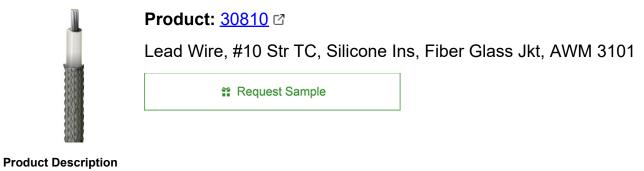
Rubber Lead Wire, 10AWG (65x28) Tinned Copper, Silicone Insulation, Fiber Glass Outer Jacket, AWM 3101 CSA SEWF-2 600V 150C
